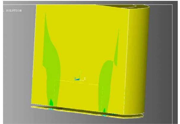
**Fig.9 Principal strains in cylinder after deformation of the membrane**
