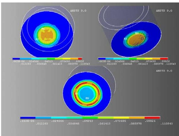
**Fig.8 Eq stress at the contact interface**
