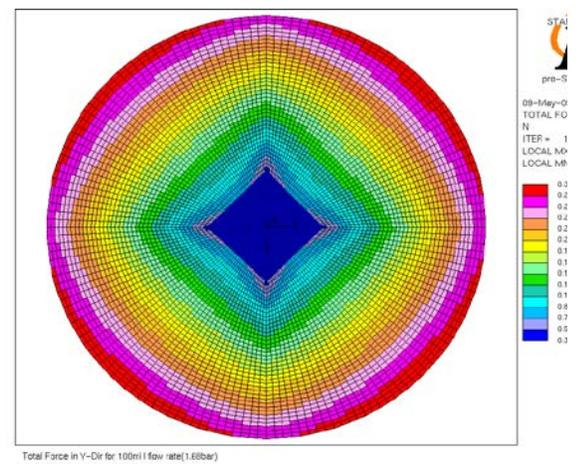
**Fig.11 Upward forces on the membrane**
