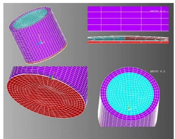
(B) Non-linear contact analysis of the assembly to ascertain the forces required to close the flow with the maximum forces
