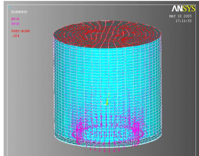
**Fig.4 B.C on contact and pressure surfaces**
