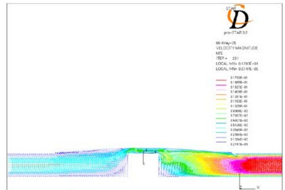
**Fig.10 Velocity vector plot in micro-channel**
