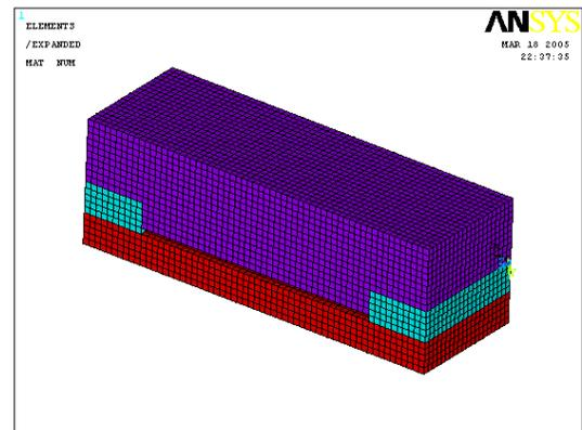
**Fig.3 Half sym model for structural Analysis**
