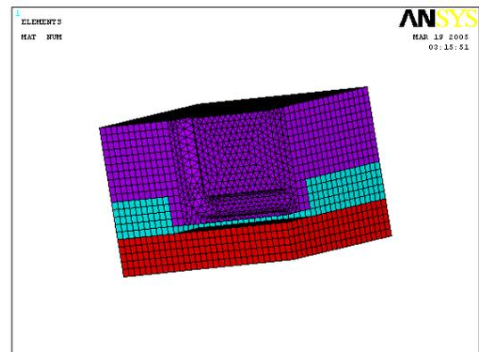
**Fig.4 Hybrid mesh for coupled analysis**
