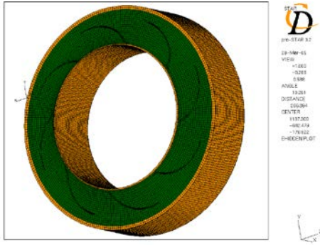
Fig 4. Fan separated and meshed
